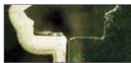
Dezincification No dezincification
