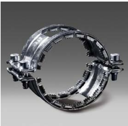
Düker Kombi grip collar Security collar with axial restraint for all Rapid, CV and CE couplings at more than 0.5 bar internal pressure
