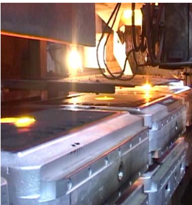
Moulding plant: pouring into the sand moulds
