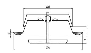
Ød = entry depth / internal diameter of a duct
