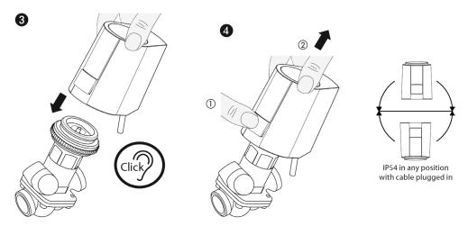
Place the actuator vertically on the valve adapter. The actuator snaps onto the valve adapter with a "click" when pressed down vertically by hand.
