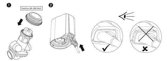
Screw the valve adapter manually onto the valve and connect cable and actuator.
