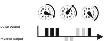
Reverse volume pulses are compensated by identical number of forward pulses before continuing with output pulses.
