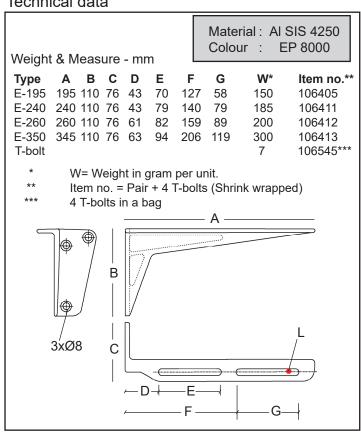
**DEFA Alu-brackets** are delivered in pairs (left and right) shrink wrapped, including 4 T-bolts.
